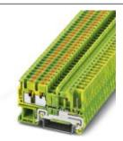
Ground modular terminal block, connection method: Push-in / plug connection, number of connections: 3, cross section: 0.14 mm² - 4 mm², AWG: 26 - 12, width: 5.2 mm, height: 35.2 mm, color: green-yellow, mounting type: NS 35/7,5, NS 35/15
