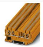
Feed-through terminal block, nom. voltage: 800 V, nominal current: 24 A, connection method: Push-in connection, number of connections: 4, cross section:0.14 mm² - 4 mm², AWG: 26 - 12, width: 5.2 mm, height: 35.3 mm, color: orange, mounting type: NS 35/7,5, NS 35/15
