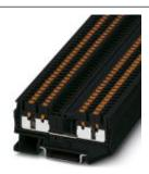
Feed-through terminal block, nom. voltage: 800 V, nominal current: 24 A, connection method: Push-in connection, number of connections: 4, cross section: 0.14 mm² - 4 mm², AWG: 26 - 12, width: 5.2 mm, height: 35.3 mm, color: black, mounting type: NS 35/7,5, NS 35/15
