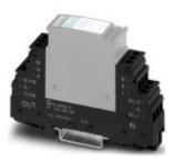
Base element to accept a protective plug with diagnostic and status indicator for one floating double wire, integrated spark gap to provide a high-resistance connection between the ground of the protective circuit of the plug and ground potential.
