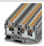
Feed-through terminal block, nom. voltage: 1000 V, nominal current: 57 A, connection method: Push-in connection, number of connections: 3, cross section:0.5 mm² - 16 mm², AWG: 20 - 6, width: 10.2 mm, height: 49.5 mm, color: gray, mounting type: NS 35/7,5, NS 35/15
