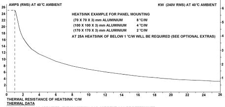
WITH HEATSINK AS SPECIFIED, THE MAXIMUM LOAD CURRENT CAN BE DETERMINED.
