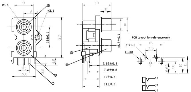
Dimensions : Millimetres Tolerance: ±0.2mm
