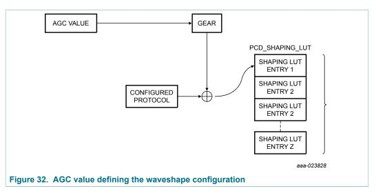
The PN5180 allows measuring periodically the RX voltage. The RX voltage is used as indicator for the actual antenna current. The voltage measurement is done with the help of the AGC. The time interval between two measurements can be configured with the OC\_TIME byte in the EEPROM.
