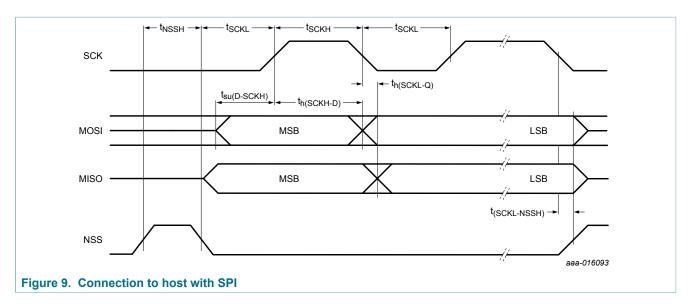
**Remark:** To send more bytes in one data stream, the NSS signal must be LOW during the send process. To send more than one data stream, the NSS signal must be HIGH between each data stream. Any data available to be read from the SPI interface is indicated by the BUSY signal de-asserted.
