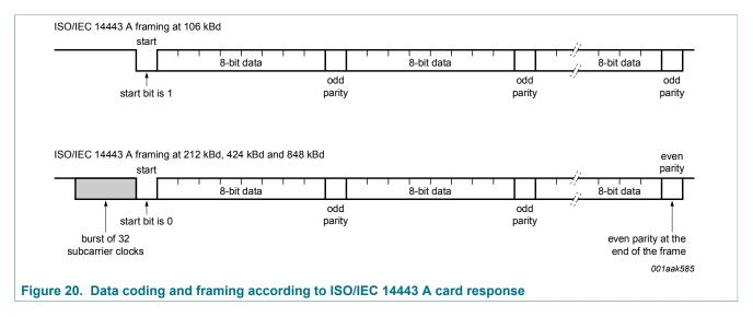
The internal CRC coprocessor calculates the CRC value based on the selected protocol. In card mode for higher baud rates, the parity is automatically inverted as end of communication indicator. The selected protocol needs to be implemented on a host processor.
