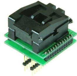
The conversion of this adapter is F:F (function to function). The adapter can be used for example for the Galep-4. With the Leaper-48 and the Superpro 3000U the adapter can only be used if the chip with the DIP24 package is selected in the respective software instead of the PLCC28 package.
