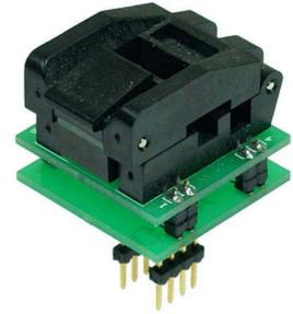
The conversion of this adapter is F:F (function to function). The adapter can be used for example for the BX32, BX32P, BX40 and Galep-4 programmers. With the Leaper-48 and the Superpro 3000U the adapter can only be used if the chip with the DIP8 package is selected in the respective software instead of the SOP14 package.
