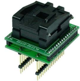
The conversion of this adapter is 1:1 (pin to pin). This adapter can be used with all chip programmers that support the desired chip.
