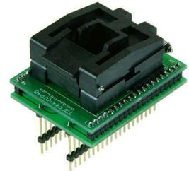
The conversion of this adapter is F:F (function to function). The adapter can be used for example for the Galep-4 programmers. With the Leaper-48 and the Superpro 3000U the adapter can only be used if the chip with the DIP40 package is selected in the respective software instead of the PLCC44 package.
