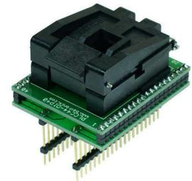
The conversion of this adapter is F:F (function to function). The adapter can be used for example for the BX40 and the Galep-4 programmers. With the Leaper-48 and the Superpro 3000U the adapter can only be used if the chip with the DIP40 package is selected in the respective software instead of the PLCC44 package.
