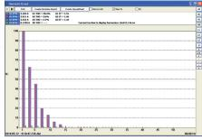
Display all harmonics from 1<sup>st</sup> to 50<sup>th</sup> in bargraph form for voltage, current and power.
