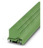
Plug component, Nominal current: 20 A, Rated voltage (III/2): 630 V, Number of positions: 1, Pitch: 7.62 mm, Connection method: Screw connection with tension sleeve, Color: green, Contact surface: Tin
