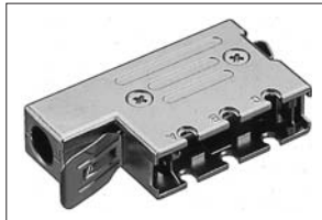
Horizontal type die-cast material backshell for standard cable with provision for preventing misinsertion PCS-E( )WSP-( )+R B-51 PCS series...49
