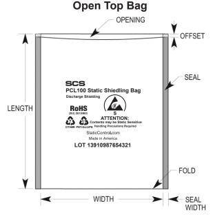
Tolerance: Width -0, +1/4" Length +/- 1/8" Offset 0 to 1/4"
