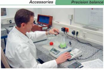
The different components of a mixture can be weighed in with the formula function. The total weight of all the components can be called up for control purposes. Documentation of the mixture is possible with the standard printers KERN YKB-01 1.
