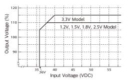
Fig.2-1 Limit of Input Voltage
