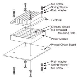
Fig.1-1 Mounting method for standard model
