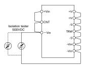
100M  $\Omega$  and above at 500VDC Fig.20-1 Isolated test
