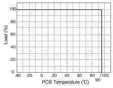
Fig.1-6 Output Derating by PCB Temperature
