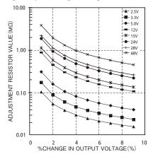
If the output voltage is raised above its nominal value, the output current needs to be derated to a value such that the output power does not exceed the maximum output power specified in the specification sheet. In addition to that, there is also a limitation to the input voltage range for the 5V version only which is as shown below.
