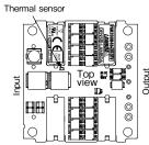
Fig.1-5 Thermal Sensor Position
