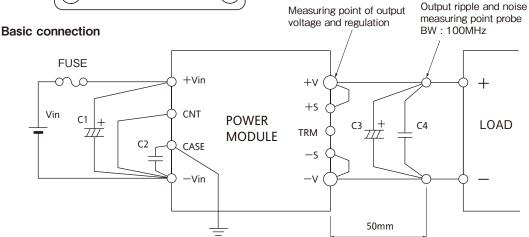
Note: This diagram is for Negative Logic "ON/OFF" Option.
