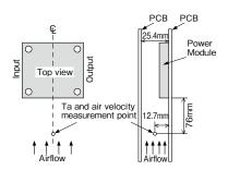
Fig.1-1 Output derating set-up condition
