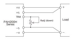
Fig.2-2 Connection for output voltage trim down (1)
