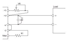
Fig.2-6 Example connection of external resistor
