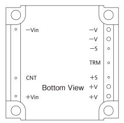
Input and Output Terminal Configurations(Bottom View)
