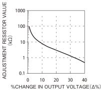
If the external resistor ( $R_{\text{adi}}$ ) is connected between the TRM pin and +S pin, the output voltage will increase. Diagram shown below is the output voltage trim up connection.
