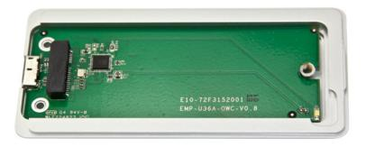
3. Insert the SSD into the black connector (see below-left). The connector is notched so that the SSD fits using only one orientation. Next, use the short Torx T5 screw to hold the SSD in place (circled below-right). Do not over-tighten the screw.
