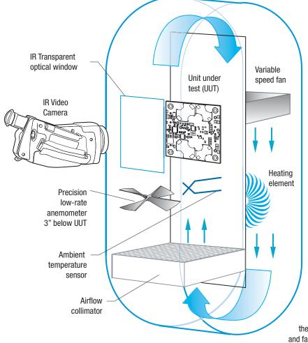
Figure 8. Vertical Wind Tunnel
