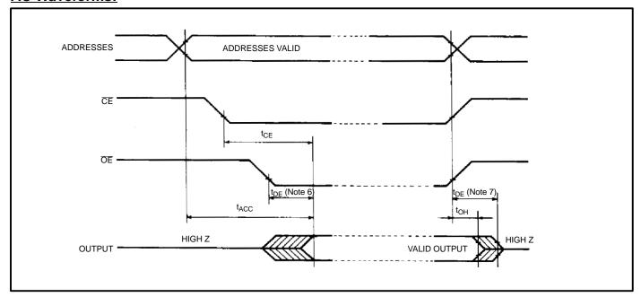
Note 6.  $\overline{OE}$  may be delayed up to  $t_{ACC} - t_{OE}$  after the falling edge  $\overline{CE}$  without impact on  $t_{ACC}$ .
