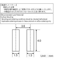
The data is reference only. Electrical characteristics vary depending on environment or measurement condition. TAIYO YUDEN reserves the right to make change to the data at any time without notice. Before making final selection, please check product specification. 2020.08.10
