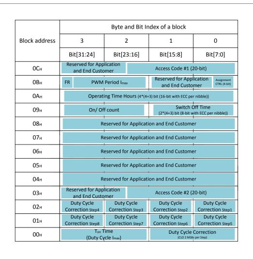
Figure 5 User Data Memory 00<sub>H</sub> to 0C<sub>H</sub>
