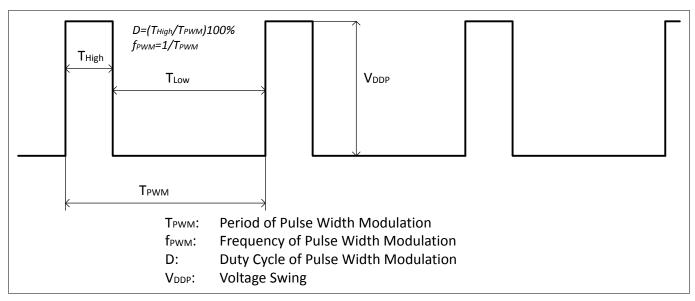
Figure 14 PWM Output Characteristics
