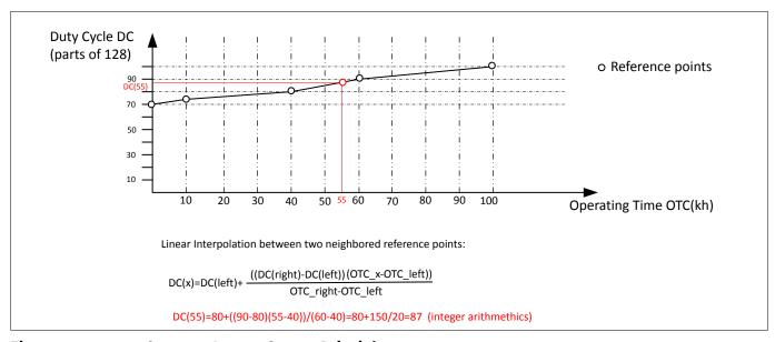
Figure 11 Constant Lumen Output Principle
