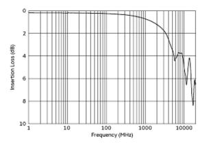
Common Mode Insertion Loss Characteristic (Typical Value)
