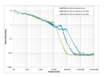
Figure 16. Noise – FIX – 5.0 V,  $I_{OUT}$  = 10 mA, Different C<sub>OUT</sub>
