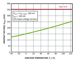
Figure 12. Dropout Voltage vs. Temperature
