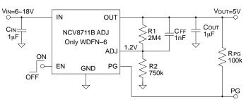
Figure 4. Adjustable Output Voltage Application with PG
