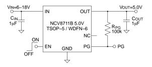
Figure 3. Fixed Output Voltage Application with PG
