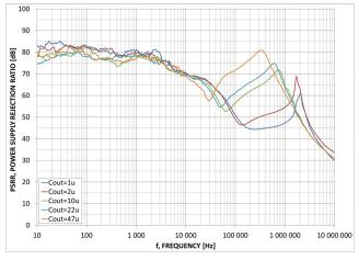
Figure 15. PSRR – FIX–3.3 V,  $V_{IN}$  = 8.3 V,  $I_{OUT}$  = 100 mA
