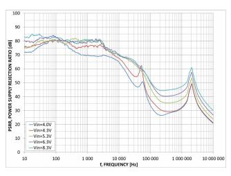
Figure 13. PSRR – FIX–3.3 V,  $C_{OUT}$  = 1  $\mu$ F, I<sub>OUT</sub> = 100 mA
