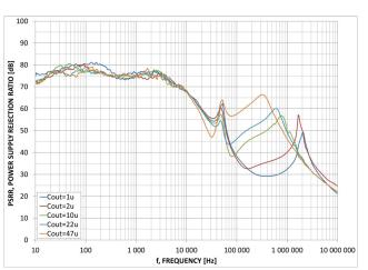
Figure 14. PSRR – FIX–3.3 V,  $V_{IN}$  = 4.3 V,  $I_{OUT}$  = 100 mA
