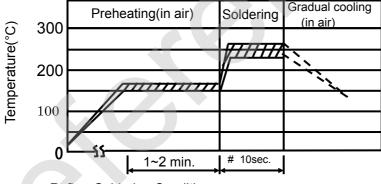
Preheating: 160 +/- 10 °C 1min. to 2 min. Soldering: 230~260°C
