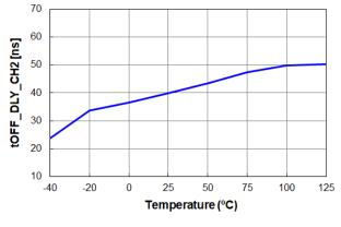
Figure 22. t<sub>OFF\_DLY\_CH2</sub> vs. Temperature
