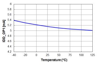
Figure 15.  $I_{DD\_OP1}$  vs. Temperature
