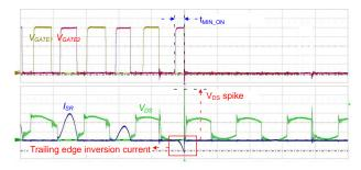
Figure 53. Trailing Edge Inversion Current
