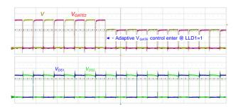
Figure 57. V<sub>GATE</sub> Control Enters when LLD is High
