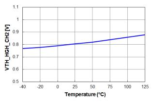
Figure 36. V<sub>TH\_HIGH\_CH2</sub> vs. Temperature
