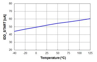
Figure 14. I<sub>DD\_START</sub> vs. Temperature
