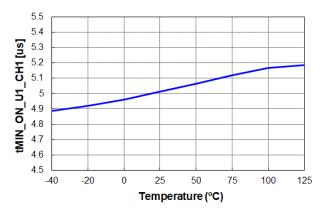
Figure 5. t<sub>MIN\_ON\_U1\_CH1</sub> vs. Temperature
