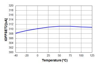
Figure 4. I<sub>OFFSET2</sub> vs. Temperature
