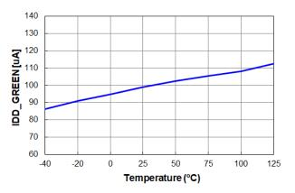
Figure 17. I<sub>DD GREEN</sub> vs. Temperature
