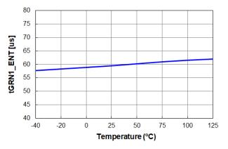
Figure 41.  $t_{GRN1\_ENT}$  vs. Temperature
