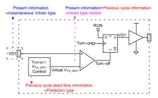
Figure 44. SR Turn-off Algorithm
