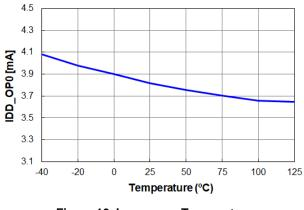
Figure 16. I<sub>DD\_OP0</sub> vs. Temperature
