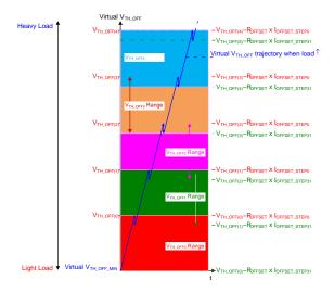
Figure 54. Virtual V<sub>TH\_OFF</sub> Trajectory when lout Increases
