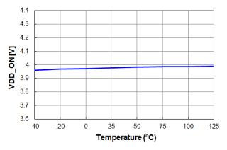
Figure 11.  $V_{DD\ ON}$  vs. Temperature
