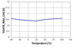
Figure 28. V<sub>GATE\_MAX\_CH2</sub> vs. Temperature
