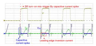
Figure 52. Leading Edge Inversion Current
