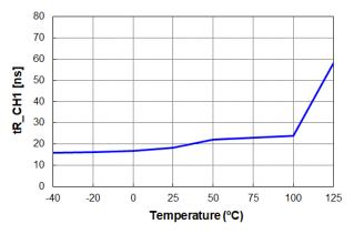
Figure 31.  $t_{R\_CH1}$  vs. Temperature
