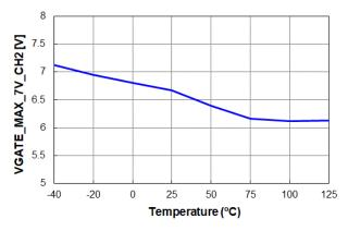
Figure 30. V<sub>GATE\_MAX\_7V\_CH2</sub> vs. Temperature
