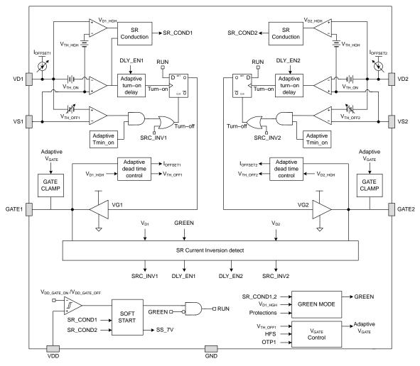
Figure 2. Internal Block Diagram of NCP4318
