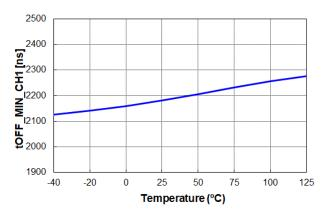
Figure 37. t<sub>OFF\_MIN\_CH1</sub> vs. Temperature
