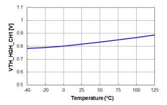
Figure 35.  $V_{TH\_HIGH\_CH1}$  vs. Temperature
