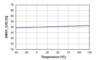
Figure 26. KINV1\_CH2 vs. Temperature
