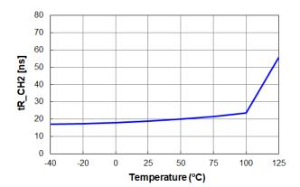
Figure 32.  $t_{R\_CH2}$  vs. Temperature
