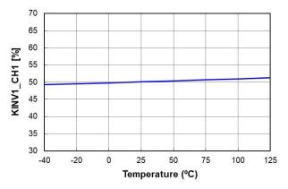
Figure 25. KINV1\_CH1 vs. Temperature
