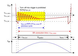
Figure 49. Minimum Turn-on Time and Turn-off
