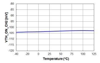
Figure 8.  $V_{TH\_ON\_CH2}$  vs. Temperature
