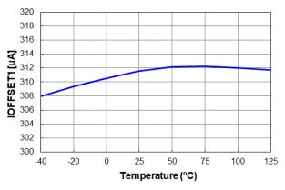
Figure 3. I<sub>OFFSET1</sub> vs. Temperature
