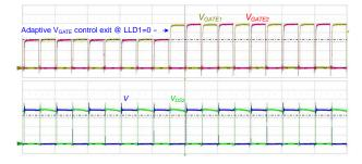
Figure 58. V<sub>GATE</sub> Control Exits when LLD is Low
