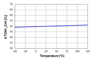
Figure 23. KTON1\_CH1 vs. Temperature
