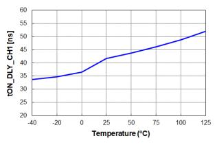
Figure 19.  $t_{ON\_DLY\_CH1}$  vs. Temperature
