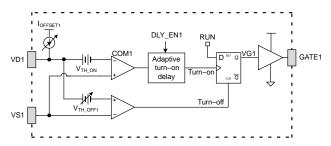
Figure 43. SR Turn-on Algorithm
