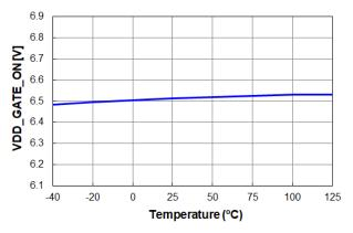
Figure 13.  $V_{DD\_GATE\_ON}$  vs. Temperature
