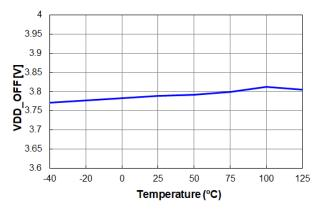
Figure 12.  $V_{DD\_OFF}$  vs. Temperature
