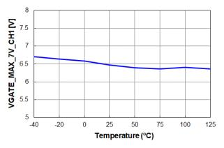
Figure 29. V<sub>GATE\_MAX\_7V\_CH1</sub> vs. Temperature
