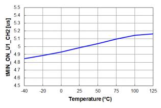
Figure 6.  $t_{MIN\_ON\_U1\_CH2}$  vs. Temperature
