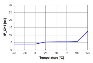
Figure 33.  $t_{F\_CH1}$  vs. Temperature
