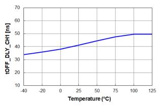
Figure 21.  $t_{\mbox{OFF\_DLY\_CH1}}$  vs. Temperature
