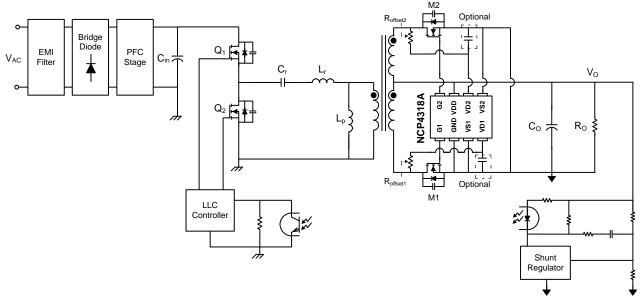
Figure 1. Typical Application Schematic of NCP4318
