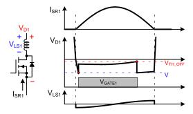
Figure 45. Premature SR Turn-off by Stray Inductor
