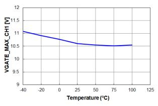
Figure 27.  $V_{GATE\_MAX\_CH1}$  vs. Temperature
