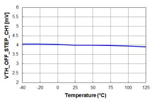
Figure 9.  $V_{TH\_OFF\_STEP\_CH1}$  vs. Temperature
