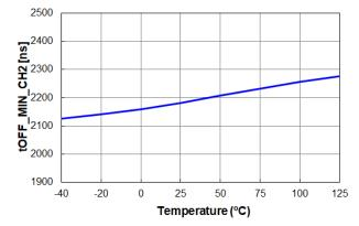
Figure 38.  $t_{OFF\_MIN\_CH2}$  vs. Temperature
