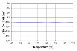
Figure 7.  $V_{TH\_ON\_CH1}$  vs. Temperature
