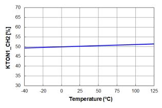
Figure 24. KTON1\_CH2 vs. Temperature
