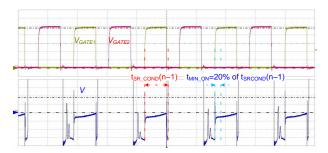
Figure 51. Minimum Turn-on Time  $t_{MIN\_ON}$  when DLY EN = 1
