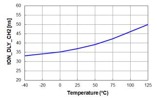
Figure 20.  $t_{ON\_DLY\_CH2}$  vs. Temperature
