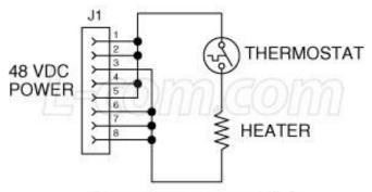
Pins 1, 2, 4, 5: + 48 VDC Pins 3, 6, 7, 8: - 48 VDC
