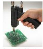
Through hole desoldering with the MX-DS1 hand-piece.
