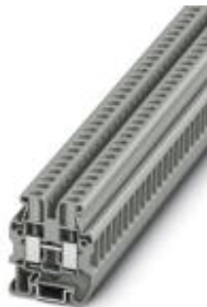
Mini feed-through terminal block, Connection method: Screw connection, Number of positions: 1, Cross section: 0.2 mm 2 - 6 mm 2 , AWG: 24 - 10, Width: 6.2 mm, Color: gray, Mounting type: NS 15
