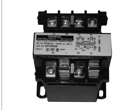
Industrial Control Power Transformers are specifically designed and built to provide adequate voltage to the load while accommodating the high current levels present at inrush. These transformers deliver excellent secondary voltage regulation and meet or exceed the standards established by NEMA, ANSI, UL and CSA. Their rugged construction and excellent electrical characteristics ensure reliable operation of electromagnetic devices and trouble-free performance.
