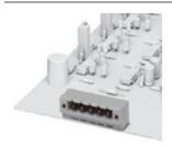
PCB headers, nominal current: 12 A, number of positions: 5, pitch: 5.08 mm, color: Agate gray, contact surface: Gold, mounting: Wave soldering, Gold-plated contact surface / color: Gray RAL 7038
