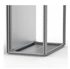
**Description:** Creates an installation surface over the full width of the enclosure. Easy installation by use of sliding profiles MTS from the side. Nominal width equals the enclosure width. When combining enclosures the MPWs can be connected and slid in as one installation surface. Can not be mounted in the rearmost position.
