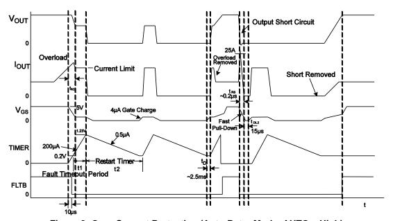
Figure 3: Over-Current Protection (Auto-Retry Mode, AUTO = High)
