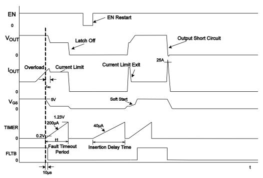
Figure 2: Over-Current Protection (Latch-Off Mode, AUTO = Low)
