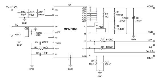
**Figure 7: Typical Application Circuit**
