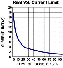
Figure 5: RSET vs. Current Limit
