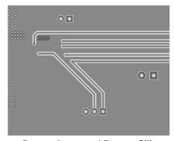
Bottom Layer and Bottom Silk Figure 6: Recommended PCB Layout
