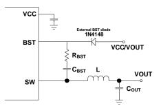
Figure 6: Optional External Bootstrap Diode to Enhance Efficiency
