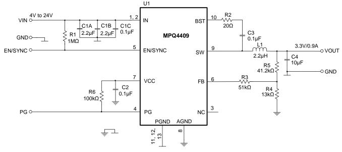
Figure 8: Typical Application Circuit, Vout = 3.3V, Iout = 900mA
