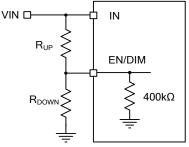
Figure 5: Adjustable UVLO using EN Divider
