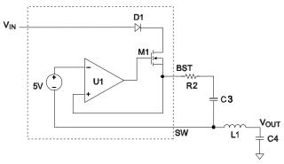
Figure 3: Internal Bootstrap Charging Circuit
