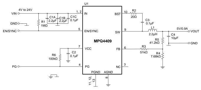
Figure 9: Typical Application Circuit, Vout = 5V, Iout = 900mA
