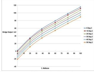
The responses exhibit a quadratic behavior and tests have shown that a 3 point calibration at 0, ~40 & 100% Methane will generate factors which will meet the requirements of EN60079-29-1 2007 part 5.4.3.2 i.e. within ±3% Methane or ±5% of indication.
