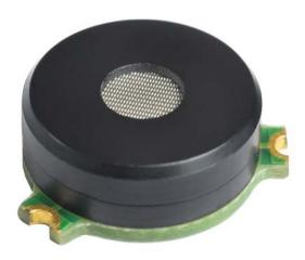
This compensator is made in the same way as a detector device except that instead of incorporating a catalyst in the coating layer, the device is treated so that oxidation cannot take place.
