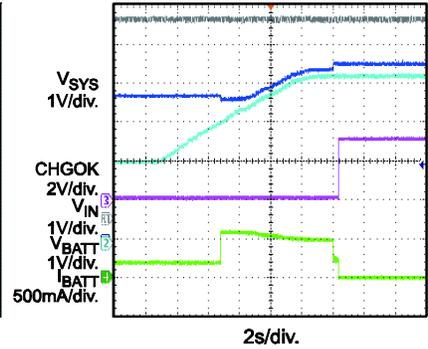
**USB IN Battery Charge Curve**
