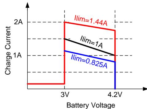
**Figure 3:  $I_{CHG}$  Variation with Different Input Current Limit**
