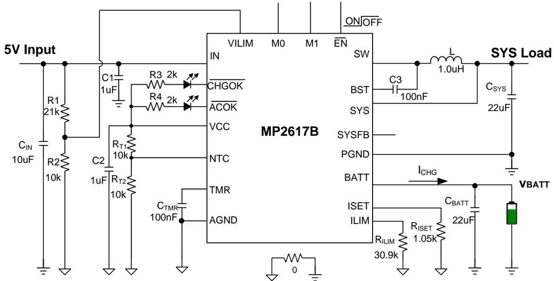
**Figure 9: Typical Charge Application Circuit for 5V input with NTC Resistor Fixed**
