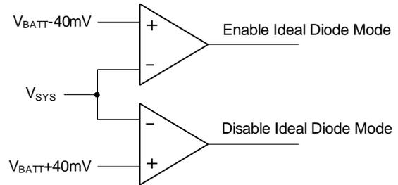
**Figure 3— Ideal Diode Mode Enable/Disable Logic Control**
