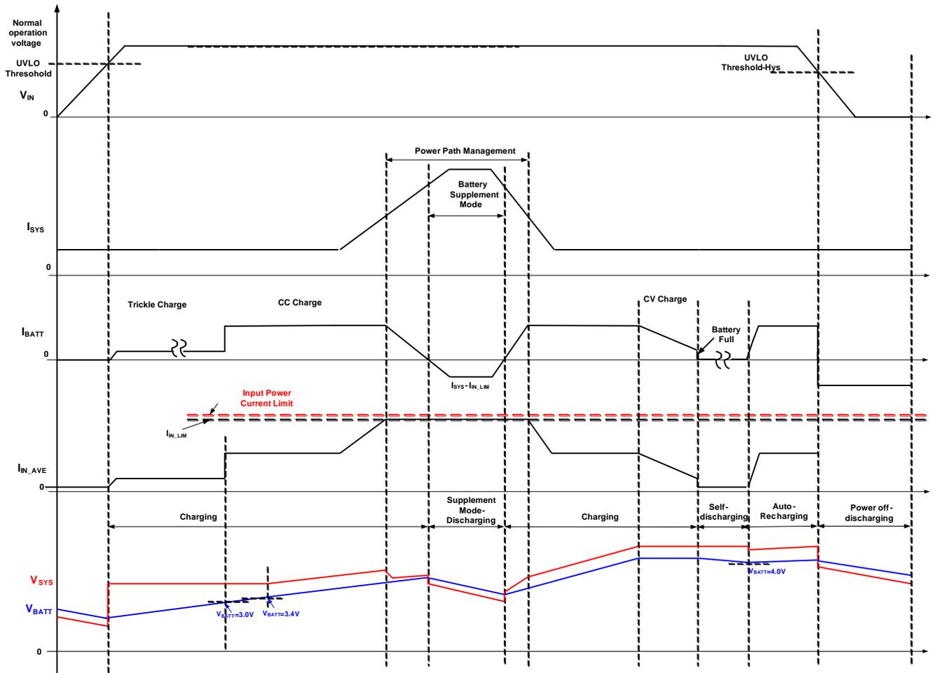
**Figure 6: MP2617B Operation Process under No Fault Condition**
