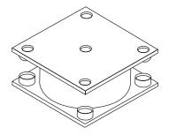
Tightening torque 20Nm max.
