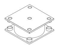
Tightening torque 20Nm max.
