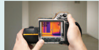
Infrared cameras quickly locate moisture related problems
