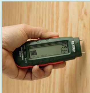
Quick measurement of Moisture levels on wood and building materials.
