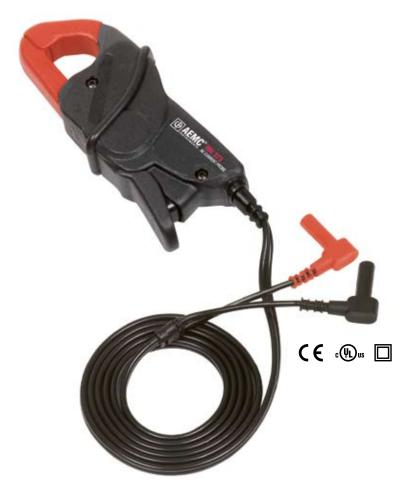
The Model MN373 is the latest in compact AC current probes. It is designed to meet the most stringent demands in industry and electrical contracting. Model MN373 meets EN 61010, 600V, Cat. III safety standards and is CE Marked and UL approved for Canada and United States.
