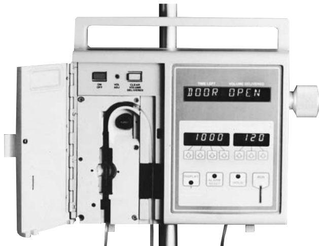
MML medical application. Intranavenous fluid flow controller automatically dispenses fluids for medications, therapy, and nutrition.
