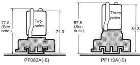
Note: PF083A(-E) and PF113A(-E) allow either track or screw mounting.
