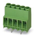
PCB terminal block, nominal current: 41 A, pitch: 6.35 mm, number of positions: 6, connection method: Screw connection with tension sleeve, mounting: Wave soldering, conductor/PCB connection direction: 0 °, color: green
