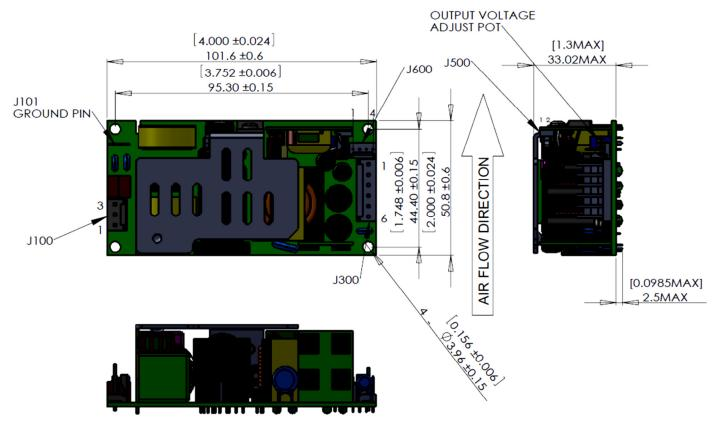
When installing the power supply into the end-product, a non-conductive Insulator should be placed between the unit and any conductive metal chassis or mounting platform.
