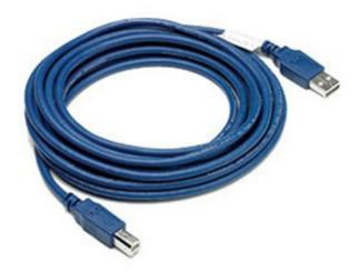
The MI121 is a high-quality, extra long 4.5 metre USB 2.0 cable, designed and built specifically for use with PicoScope oscilloscopes, and featuring 20-AWG conductors for minimal resistance. This also reduces the chance of voltage drop caused by inferior USB ports on some PCs and laptops. As well as reducing voltage drop, it prevents noise that could be caused by an unreliable ground connection and poor screening in inferior cables.
