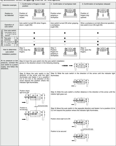
Note 1) It is recommended that gripping of a workpiece be performed close to the center of the finger stroke.
