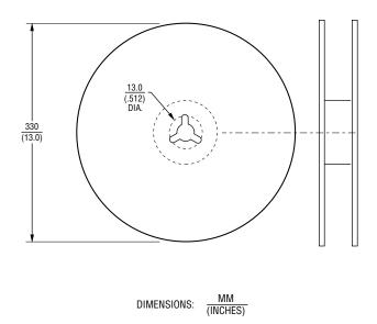
\*Bulk packaging is standard for Model MF-LR Series; consult factory for tape and reel option.
