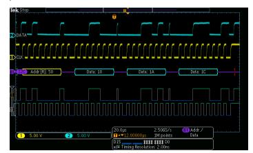
Triggering on a specific address and data packet going across an I<sup>2</sup>C bus. The yellow waveform is clock and the blue waveform is the data. A bus waveform provides decoded packet content including Start, Address, Read/Write, Data, and Stop.
