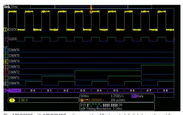
The MDO3000 with MDO3MSO option provides 16 integrated digital channels enabling you to view and analyze time-correlated analog and digital signals.
