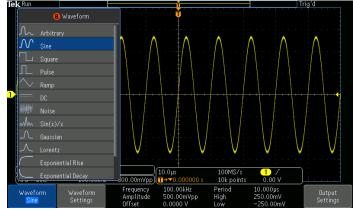
Waveform type selection in the integrated AFG.
