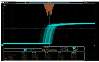
Waveform histogram of a rising edge showing the distribution of edge position (jitter) over time. Included are numeric measurements made on the waveform histogram data.
