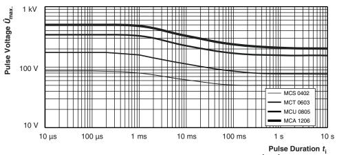
Maximum pulse voltage, single and continuous pulses; applicable if  $P \leq P_{\text{max}}$ ; for permissible resistance change equivalent to 8000 h operation in standard operation mode
