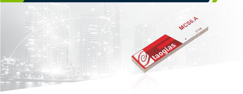
The MCS6.A is a low profile SMD NB-IoT / CAT M1 Bands / 4G/3G/2G embedded antenna designed for direct SMD mount on a device PCB. It provides high efficiency in a very small form factor of just 42\*10\*3mm.
